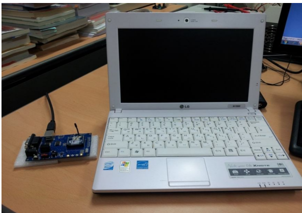
Fig. 1. XBee connected to PC via Xbee interface board.
